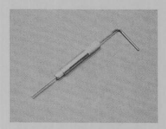
If adjusting the trim screw does not bring the CO level into specification, adjust the mixture needle. This requires a special tool.
