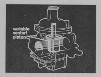
Now, a variable venturi piston is added. The action of the throttle plate controls the position of the piston which varies the venturi size (or opening).
