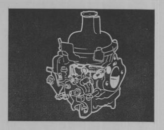
Another emission reducing device found on some versions is a vent valve. The vent valve controls the fuel bowl venting, which, in turn, is controlled by the throttle position.
