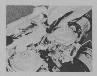
Blow into the hose again. If no restriction is felt, the vent valve is adjusted correctly. If a restriction is felt, turn the adjusting screw counter clockwise until the restriction just disappears. This is the correct setting.
