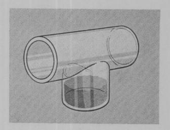
A fuel supply . . . usually in a bowl beneath the venturi;
