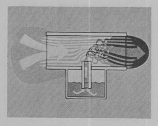
The depression draws fuel through the jet from the fuel bowl. The fuel then mixes with the fast moving air in the venturi.
