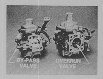
All carburetors are now fitted with a bypass valve or an overrun valve to reduce emissions on deceleration.
