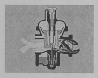
So now we have a way of metering the fuel into the venturi in relationship to the throttle position and the venturi size. This allows very precise response and smooth operation.
