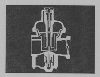
Many refinements are necessary to make this basic carburetor suitable for automobile use. All carbureted BLM cars use constant velocity variable venturi carburetors. The refinements for this type of carburetor are as follows:
