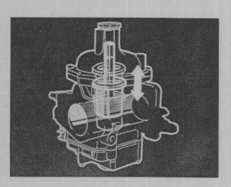
The piston moves up and down to increase or decrease the venturi size.
