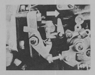
Be sure the choke is off and the fast idle cam is not in contact with the adjustment screw.
