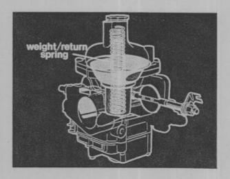
Further refinements to the basic carburetor include: A weight/return spring which helps move the piston down.
