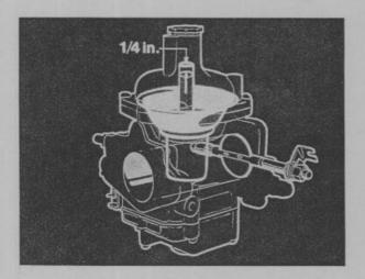
Remove the damper assembly from the top of the carburetor. Raise the piston with your finger through the carburetor opening. With the piston raised all the way, top up the damper tube with engine oil until the level is ¼ inch from the top of the tube. Then, re-install the damper assembly. Again, raise the piston all the way. This will enable you to position the oil retaining clip during installation.
