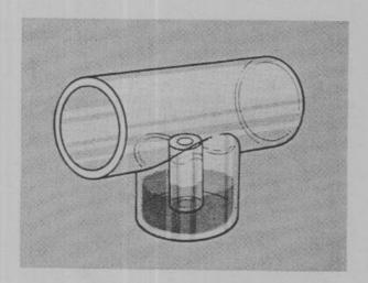
And . . . a small orifice for transferring fuel from the fuel bowl into the venturi. This is generally referred to as a jet.
