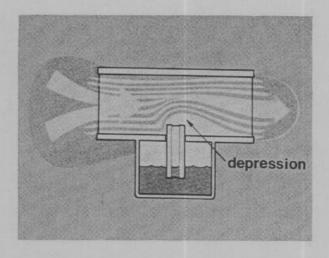
The operation is quite simple. As the engine draws air through the venturi, a low pressure area . . . or depression is created over the jet opening.
