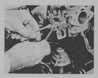
Adjust the fast idle screw and lock nut to specification. On twin carburetor installations, ensure equal air flow through each carburetor.
