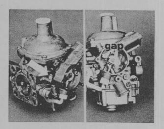
Now, turn the adjusting screw until the gap between the throttle stop and the cam is as specified. The specification can be found in your workshop manual or training aid.
