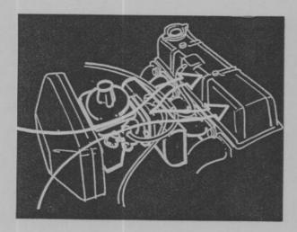
The fuel/air mixture passes into the engine's combustion chamber where it is ignited and burned to produce power. But the type of carburetor we have just illustrated would only be satisfactory if the engine were to run at one speed, however, it would not be suitable for varying engine speeds and loads . . . and would require an external starting aid to start the engine.
