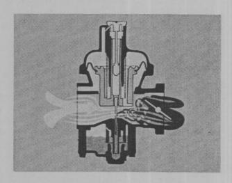
Again . . . the fuel atomizes and mixes with the incoming air. The mixture then passes into the combustion chamber where it is ignited and burned.
