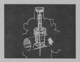
The initial upward movement of the piston is limited by the hydraulic damper. This provides initial mixture enrichment to prevent hesitation.
