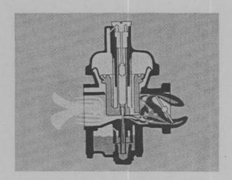
The depression over the jet draws fuel into the venturi from the fuel bowl which atomizes and mixes with the incoming air. The mixture then passes into the engine's combustion chamber where it is ignited and burned.
