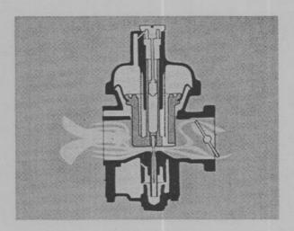
At idle, the throttle plate is partially open and a slight depression is created on the downstream side of the piston. The slight depression is channeled to the upper chamber. However the piston is only partially raised because the difference in pressure is not great enough to overcome the weight of the piston and the spring tension.
