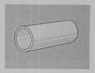
A carburetor has three essential elements: A tube for high velocity air flow called a venturi;
