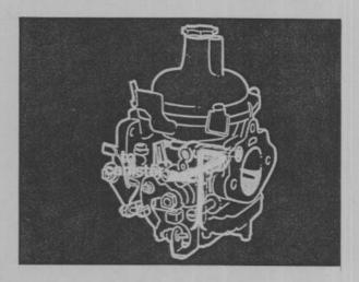
The vent valve vents the fuel bowl to the charcoal canister during idle.
