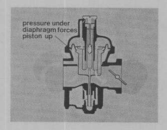
The difference in pressure causes the piston to be raised to a partially open position. This occurs because the atmospheric pressure, acting on the bottom of the diaphragm, is greater than the venturi pressure.
