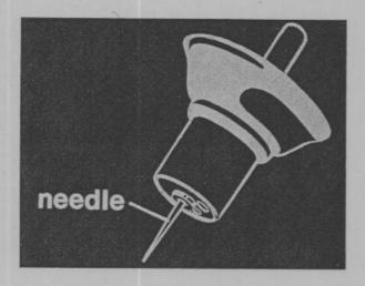
A further refinement is the tapered fuel metering needle. The needle is attached to the piston and moves up and down with it.
