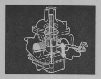
The needle taper varies the jet opening size as the needle moves up and down with the piston. This controls the amount of fuel flowing into the venturi.
