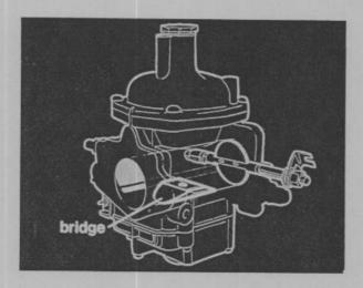
The next refinement is a bridge under the piston which creates turbulence and produces better fuel atomization. It also provides depression at full throttle.
