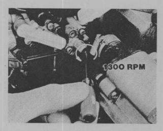
Then, turn the valve adjusting screw counter clockwise until the engine speed returns to 1300 RPM. Now, open and close the throttle. The engine speed should drop to approximately 1300 RPM when the throttle is closed. Adjust as necessary to achieve this condition.
