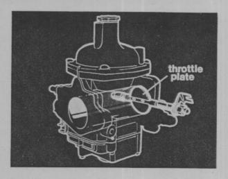
The first necessary refinement is a throttle plate. As the throttle plate is opened and closed, it controls the amount and velocity of air passing through the carburetor.
