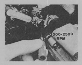
If adjustment is necessary on a single carburetor installation, begin by turning the valve clockwise until the engine speed increases abruptly to 2000 to 2500 RPM.
