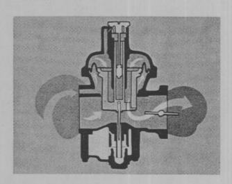
During acceleration, the throttle plate is completely open. This creates an even greater depression in the venturi and the pressure difference in the two chambers is the greatest. Remember, the venturi and atmospheric pressures are channeled to the chambers on top of the piston.
