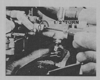
Finally, turn the valve adjusting screw one half turn more in the counter clockwise direction. Then reconnect the vacuum hose to the distributor.
