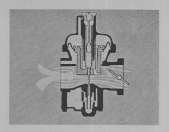
The depression over the jet is greater due to the increased air velocity. And . . . as the metering needle has moved up with the piston, more fuel flows into the venturi.
