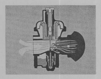
The depression over the jet becomes greater as the piston moves up and the air velocity increases. Also, the metering needle allows more and more fuel to enter the venturi as it raises with the piston. When the piston is raised all the way (open), the needle allows maximum fuel flow and the piston allows maximum air flow. The mixture passes onto the combustion chamber where it is ignited and burned producing maximum power.
