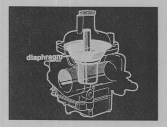
At the top of the piston, atmospheric pressure and the downstream venturi pressure are channeled into separate chambers. In the Stromberg, the chambers are separated by a diaphragm.
