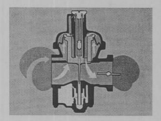
After the initial dampening, the piston gradually raises all the way, opening the venturi to its maximum size, giving a very smooth transition from low speed to high speed.
