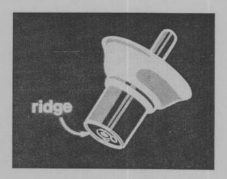
At rest, the piston does not completely cut off the venturi as it is held open by a ridge or pad at the bottom of piston. This allows starting and idling.
