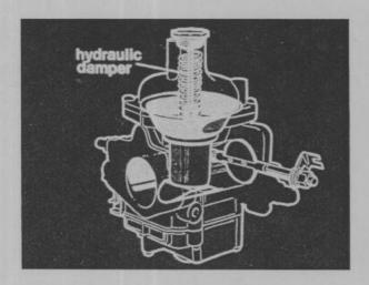
A hydraulic damper which limits the initial piston movement. This provides initial enrichment on acceleration.
