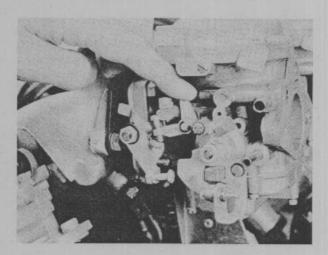
Now, blow into the hose and at the same time move the lever that operates the vent valve. As the lever is operated, a sudden restriction will be felt while blowing into the tube. This will allow you to feel the valve operation.
