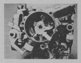
Fast idle is provided by a stepped cam and an adjusting screw. The cam and bi-metal spring use the same pivot.
