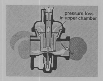
At cruise, the throttle plate is open approximately half way, causing a greater depression on the downstream side of the piston. The depression is channeled to the upper chamber, and this produces a substantial difference in pressure in the two chambers on top of the piston.
