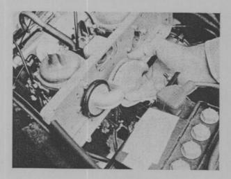
Using an air flow meter, check the air flow of each carburetor.
