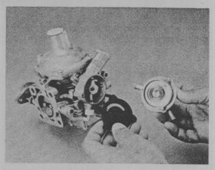
On automatic choke versions, remove the carburetors, then remove water jacket, gasket, sealing ring, and the heat mass and the insulator from the choke unit.
