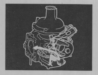
The needle moves to meter fuel into the carburetor with changes in engine coolant temperature. A bi-metal spring attached to the needle senses coolant temperature. When the temperature is low, full fuel flow is allowed. As the engine warms up, fuel flow is gradually decreased by movement of the spring and the needle. When the engine is completely warmed up, the fuel flow is cut off.
