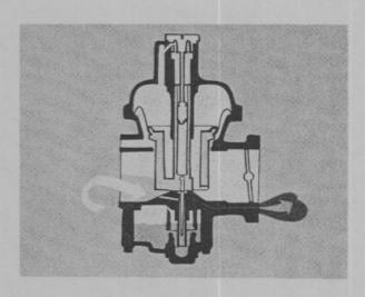
In some versions, an idle/slow run emulsion circuit replaces the temperature compensator. This is a separate circuit which discharges its mixture downstream of the throttle plate.
