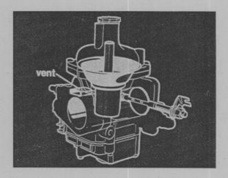
And . . . the underside of the diaphragm or upper piston is vented to the atmosphere through a drilling in the carburetor body.
