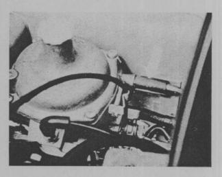
Ensure that the engine idle speed is set to the correct specification. Then, stop the engine, and remove the existing vent valve hose from the carburetor. Attach a separate piece of hose to the vent valve tube on the carburetor.
