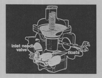
And . . . a float controlled inlet needle valve in the fuel bowl which governs the fuel level. Now we have a carburetor that is suitable for automotive use. So, let's look at how it operates . . . druing idle, cruise and acceleration.
