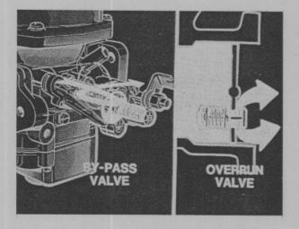
These one way, spring loaded valves, allow the mixture to bypass the throttle plate when the throttle plate is suddenly closed. The high manifold vacuum present at this time, unseats the valve and allows the mixture to flow directly into the combustion chamber.
