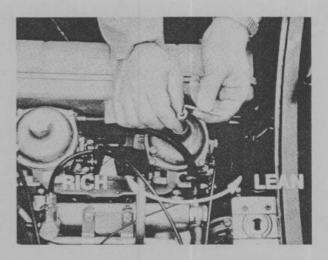
Slowly insert the special tool into the dashpot until the outer tool engages the air valve and . . . the inner tool engages the hexagon in the needle adjuster plug.
