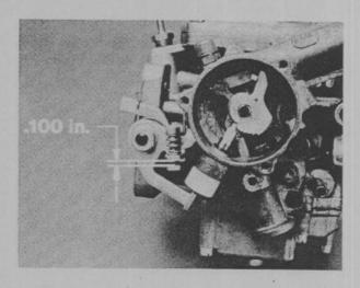
Then, set the linkage gap to a minimum of 100".
