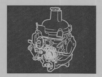
Some versions of the Stromberg carburetor use a manual choke to aid in cold starting. A separate channel is made between the fuel bowl and the low depression area of the carburetor. A disc with a series of drillings is positioned to control flow in the channel.
