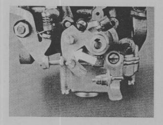
Besides mixture enrichment, the choke cable also controls the carburetor fast idle cam. This provides increased engine RPM during warmup.
