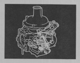
Other versions of the carburetor use an automatic choke, which also has a separate channel from the fuel bowl to the low depression area of the carburetor. However, fuel flow is controlled by a jet and needle. The jet is in turn controlled by a bi-metal strip.
