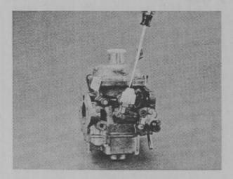
First, adjust the fine mixture trim screw. If twin carburetors are fitted, adjust both carburetors in equal amounts.
