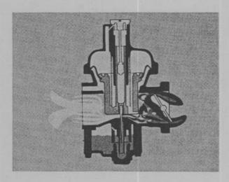
This weakens the depression and the piston falls slightly. The fuel supply is reduced by the lowering of the needle and this creates a leaner mixture.
