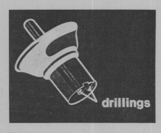
The downstream side of the piston is vented to the top of the piston by two drillings in the piston itself.
